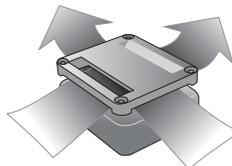
Sandwich webbing between retractor & bracket (either horizontally or vertically). Screw bracket to retractor
